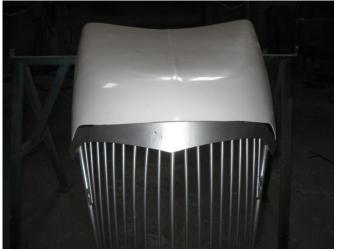
WHEN MOUNTING THE 37 CHEVROLET HOOD / GRILL, THE FRONT EDGE OF THE HOOD WILL MATCH UP WITH THE TOP EDGE OF THE GRILL. (THE HOOD SHOULD NOT OVERLAP THE GRILL)
