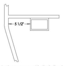
Note: The measurement for the battery box offset will be taken at the point closest to the crossmember, from the inside of the framerail to the otside of the battery box.
